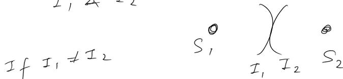
(i)  $I = I_1 + I_2 + 2 \sqrt{I_1} \sqrt{I_2} \cos \phi$   $\phi = \Delta \phi$  (Phase diff. b/w 2 waves  $y_1$  &  $y_2$ )
