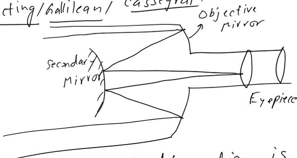
\* Chromatic Aberration is nullified using reflecting telescope.
