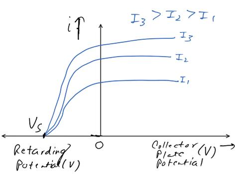
Note:- Stopping potential is independent of intensity of light & is dependent on frequency of light only.
